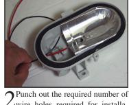
2 Punch out the required number of wire holes required for installation. Three holes are provided. Holes are scaled for 1/2" conduit. Insert positive and negative wires.
