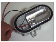
Punch out the required number of wire holes required for installation. Three holes are provided. Holes are scaled for 1/2" conduit. Insert positive and negative wires.
