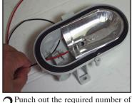
2 Punch out the required number of wire holes required for installation. Three holes are provided. Holes are scaled for 1/2" conduit. Insert positive and negative wires.
