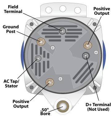
Terminal connections on Balmar 98-24-220-BL-IG are shown. Terminal locations may vary on other 24-volt alternators. See alternator manual
