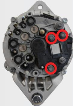
*Remove the Back Cover (2 screws)
