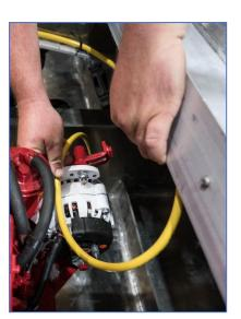
The photograph to the right represents a good installation of the battery negative cable. The cable is run with chafe protection and is secured to the engine with a cable tie (see the yellow circle) a short distance from the alternator.
