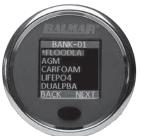
The currently selected battery type is noted with an asterisk (\*) in front of the name. The default is FLOODLA (see the chemistry table). If this is your chemistry and the installation is new, you may either re-select the chemistry, ensuring that the SG200 is starting fresh, or exit back to MENU and move to the next step.
