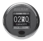
Once you select a chemistry, you must specify the capacity of the battery bank. This is the total design capacity of the entire bank, regardless of the battery's condition, or previously measured capacity. Typically the capacity is expressed as the 20-hour discharge rate. This may be written as something like "105Ah/20h" on the battery or battery documentation. If you cannot find
