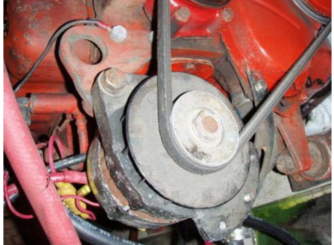
18. Once the new water pump is installed, remove the old alternator from its mounts.
