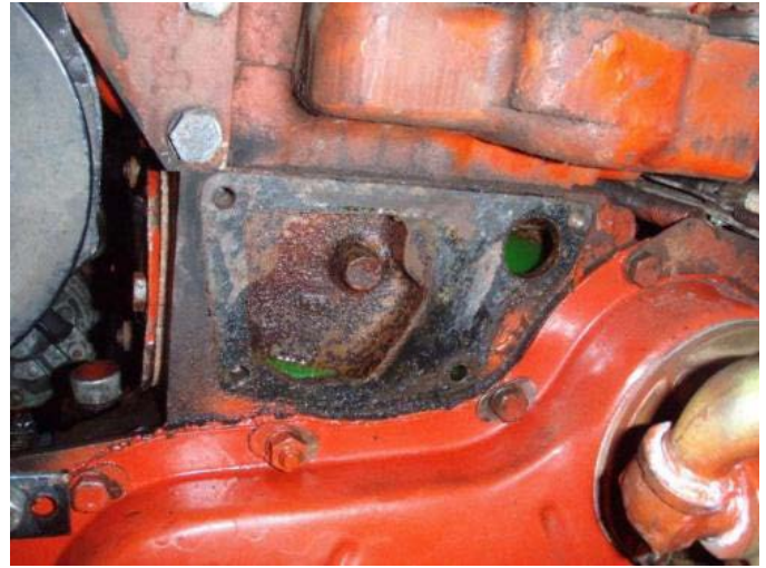
15. The surface of the engine block must be thoroughly cleaned and smooth before the installation of the new pump.
