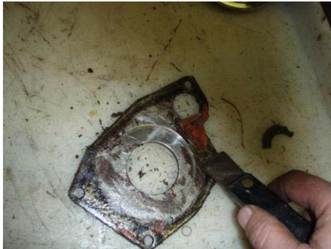
16. The gasket plate must be free of any old sealants or any other foreign matter before re-installation. Don't take any shortcuts during this process.
